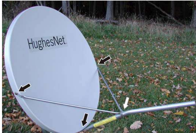
Figure 19: Tightening nuts on support rods and feed support arm
