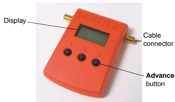
Figure 43: DiSEqC Antenna Pointing Tool (DAPT)
