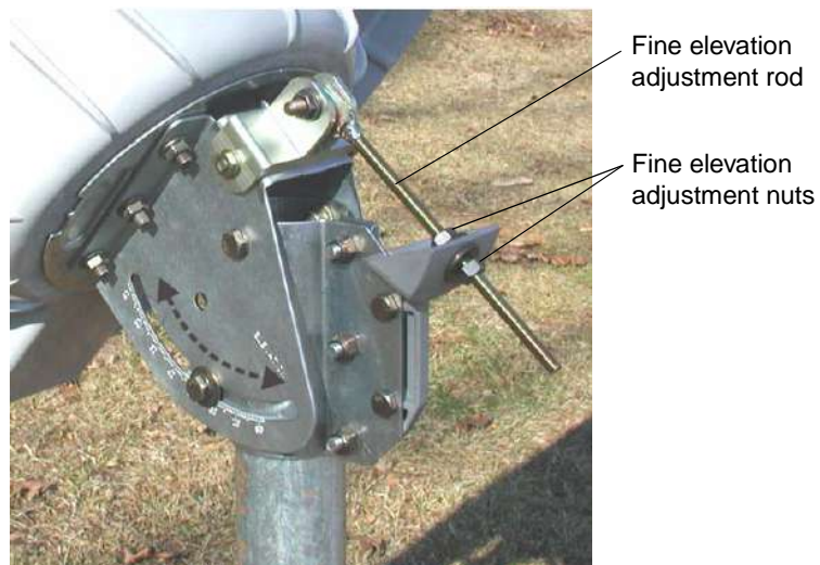
Figure 50: Fine elevation adjustment
