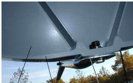
Back of reflector Rim Flat end of feed support arm
