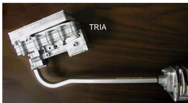
TRIA rotated for vertical polarization
