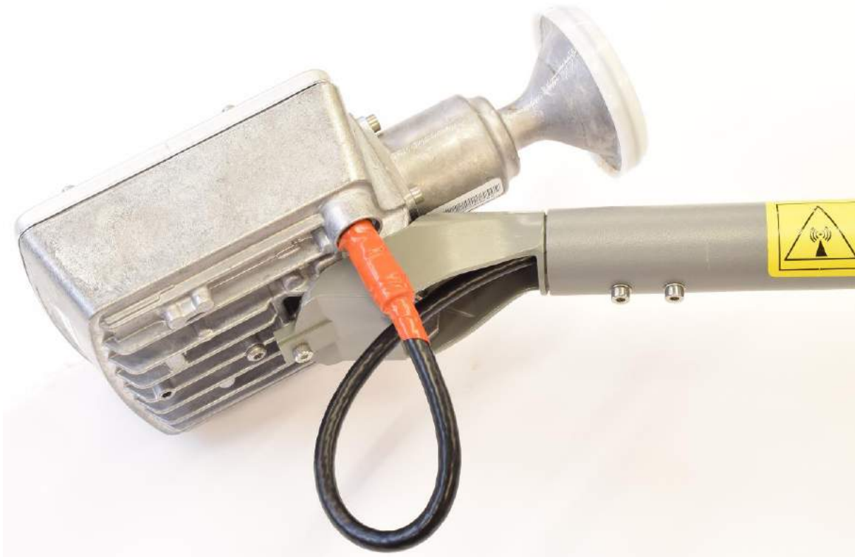
Figure 31: Hughes-approved IFL cable connector with additional weatherproofing
