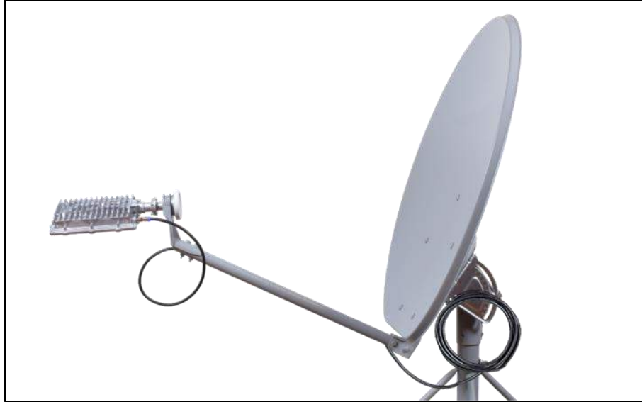
Figure 25: IFL cable configuration (shown with single IFL radio)
