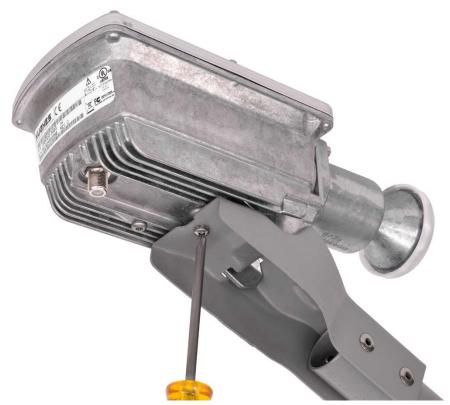
Figure 15: Securing the radio
