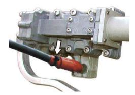
Figure 37: Weatherproofed connection with cable tie (arrow)
