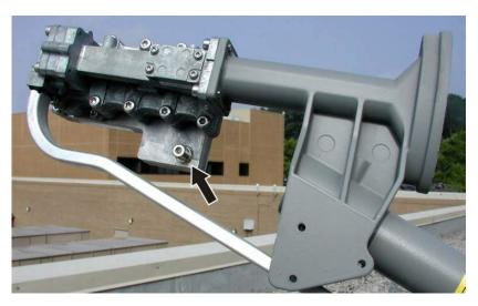
Figure 25: Receive connector
