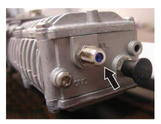
Figure 24: Transmit connector
