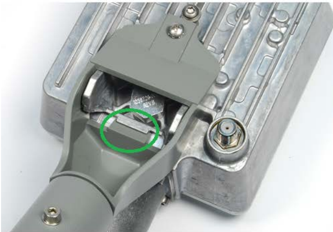
Correct Toothed notch fits under radio slot
