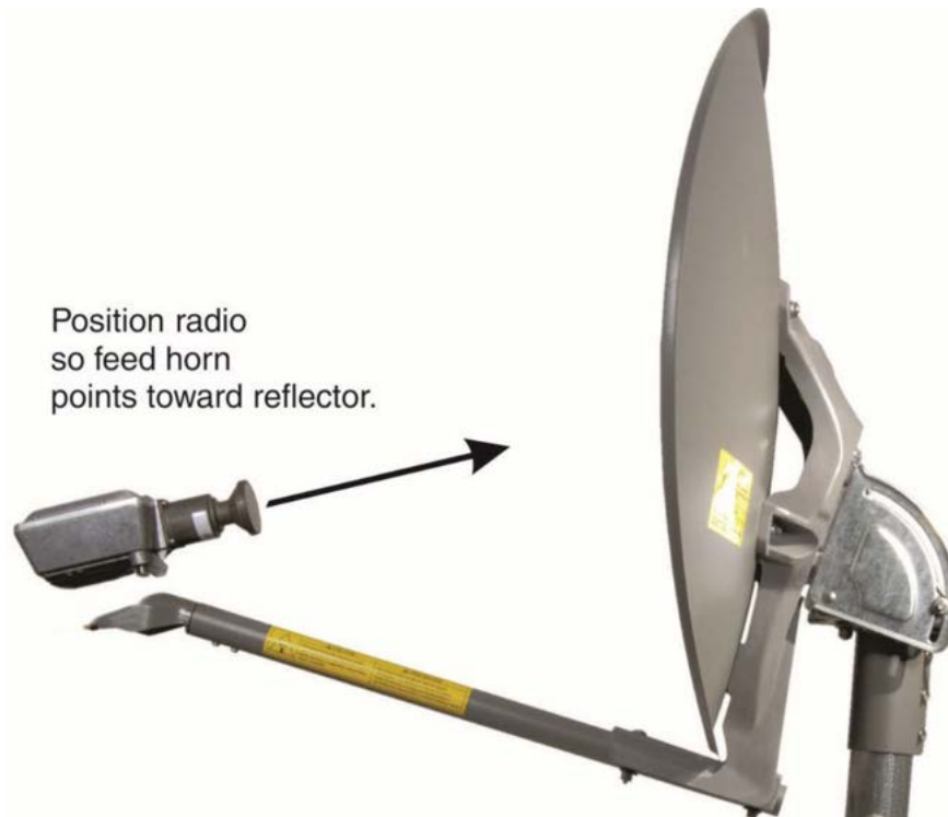
Figure 12: Radio position on antenna assembly
