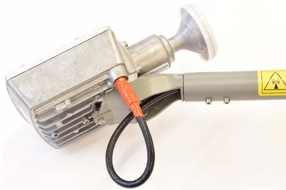
Figure 28: Hughes-approved IFL cable connector with additional weatherproofing
