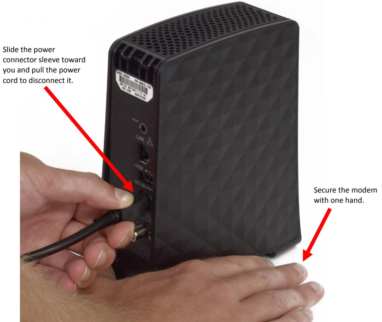
Figure 5: Disconnecting the power cord from the modem
