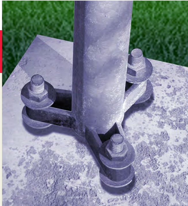
ANCHOR PATTERN 1 96 cm - 1.2 m (3) 3/4" Anchors Equally Spaced on 6.80" Bolt Circle
