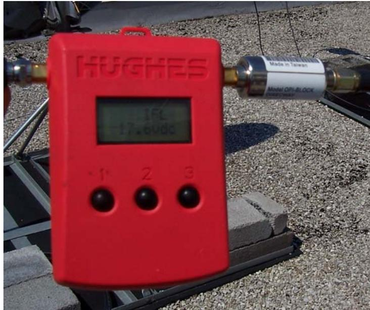
Once the DAPT and filter are correctly assembled and installed, the first thing to notice is the displayed information. It will be showing you the actual voltage on the Rx IFL cable. This value could be anywhere between ~12.6vdc and as high as ~18.2vdc. This is based on Horizontal or Vertical receive of the system.
