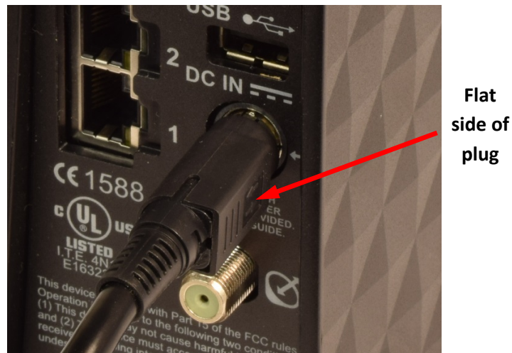
Figure 6: Proper power cord orientation
